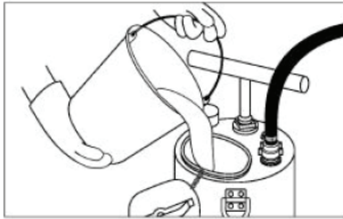
Figure 18: Add the right amount of water and insecticide in the spray can
