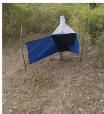
Figure 35: Setting and deployment of Ngu trap
