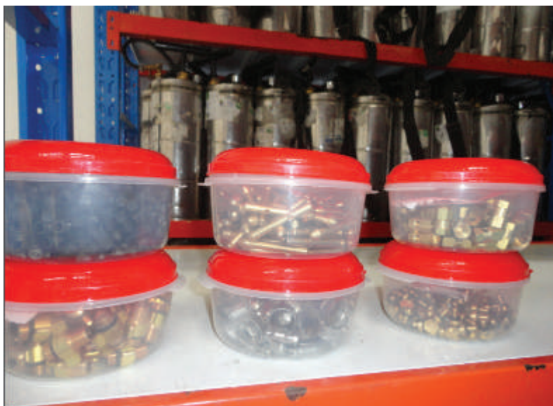
Figure 17: Spray pump spare parts arranged in plastic container
